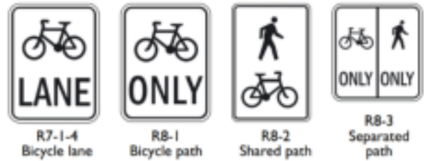
▲ Regulatory signage for general on and off-road bicycle facilities
