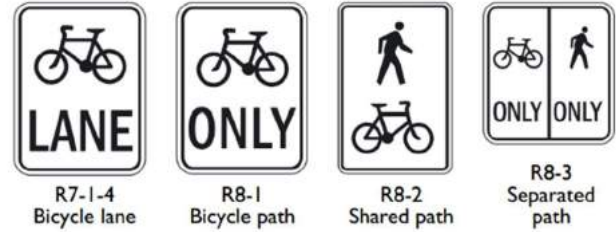
▲ Regulatory signage for general on and off-road bicycle facilities
