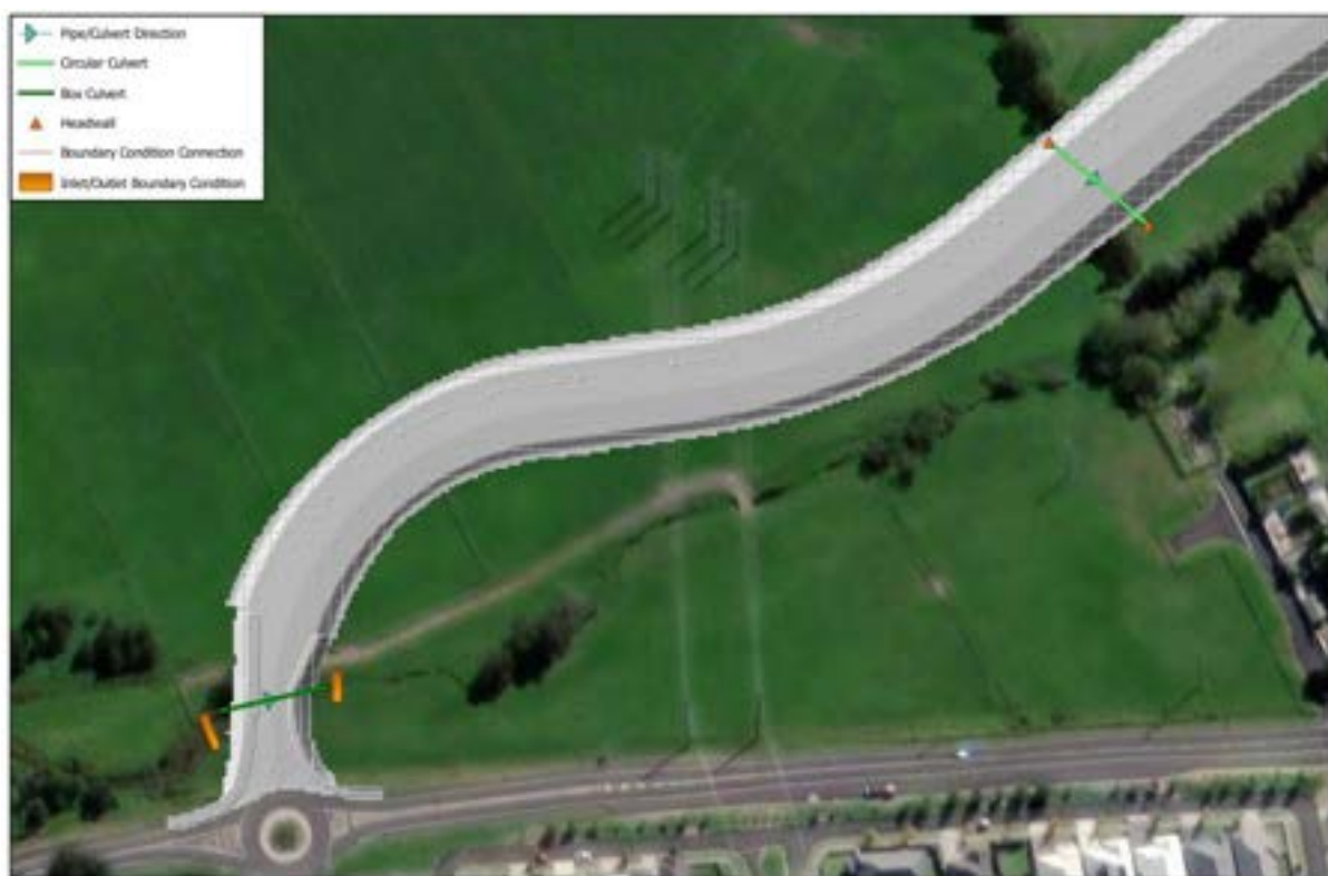
Figure 2-3 Hydraulic Structures Upstream Culvert
